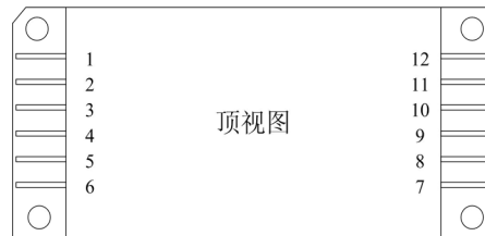
Figure 2 Diagram of the lead end arrangement
