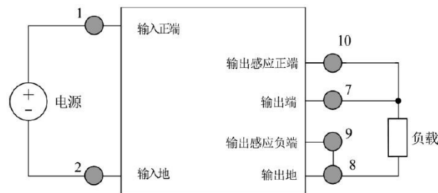
Figure 6 Connection diagram of the sensing end
