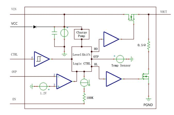
N-mosfet Integrated for High side and Low side Charge Pump Inside supporte Continuous Mode
